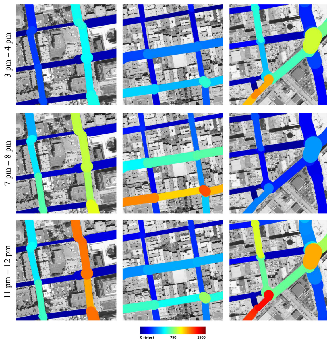
Fig. 14 Visualization of taxi traffic at three different locations in San Francisco city. Columns and rows correspond to locations and time intervals, respectively. The number of taxi trips is indicated by different colors on road regions, which is superimposed on the gray-level aerial
